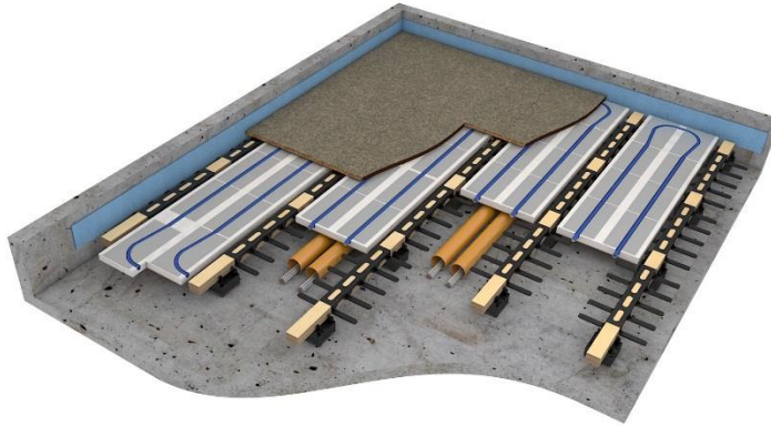
Construction LD-01 – 18mm chipboard substrate – budget substrate for floor finishes such as carpet, engineered-timber floorboards, lino, marmoleum
